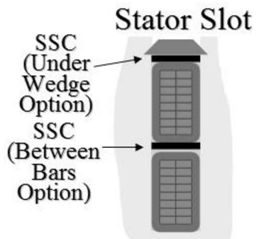
SSCs Installed in Stator Slots of Turbo-Generator
